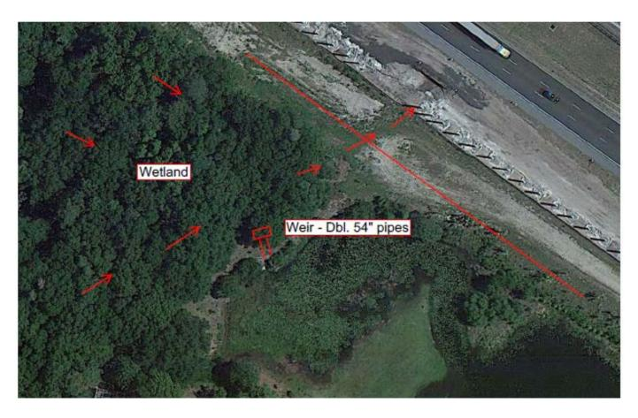
Prepared By FDOT August 2012This Schematic Depicts Watershed Flow From TPOST 3 Under I 75 – In Direction of Trout Creek
