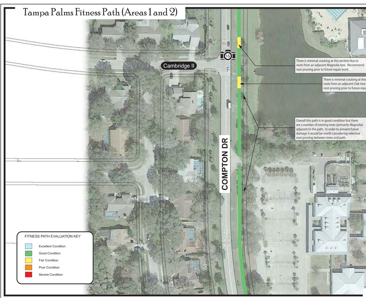
SCALE: 1" = 80'-0" so. A 1-15 There is minimal cracking at this section due to roots from an adjacent Oak tree. Recommend root pruning prior to future repair work. leeart
