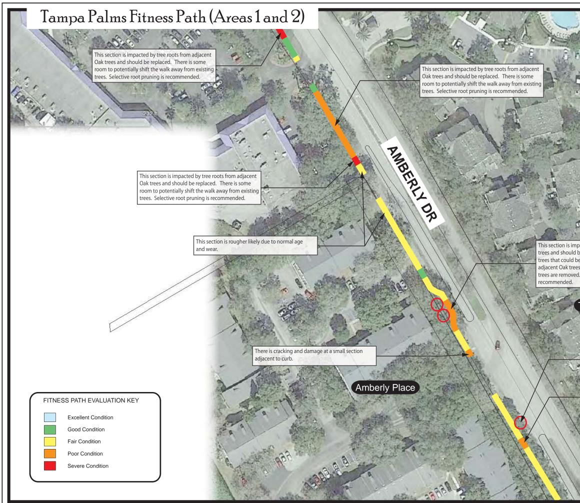
This section is impacted by tree roots from adjacent trees and should be replaced. There are (2) two Elm trees that could be considered for removal. There are adjacent Oak trees that can infill gap in canopy if these trees are removed. Selective root pruning is
