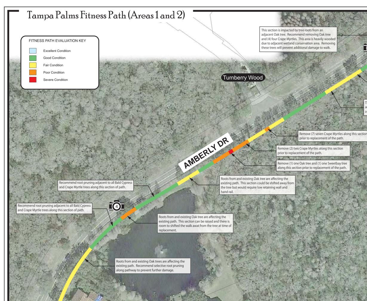
This section is impacted by tree roots from an adjacent Oak tree. Selective root pruning or removing the tree is recommended prior to repair.
